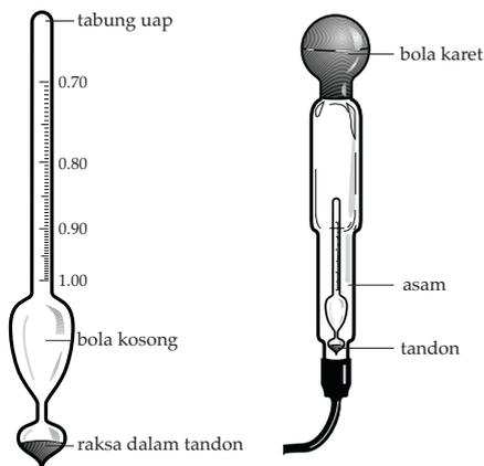
Gambar 14.25 Hidrometer
