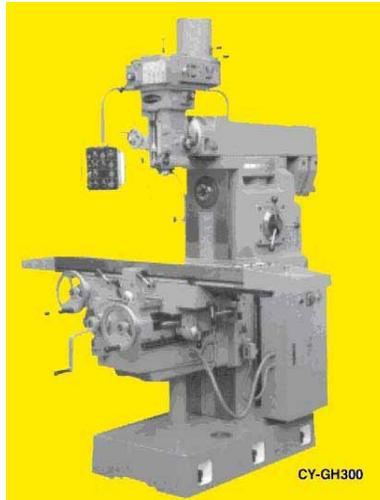
Gambar 7 2. Mesin Frais *turret vertical horizontal*.
