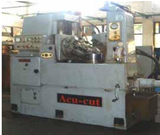
Gambar 86. Mesin frais roda gigi ( gear hobbing machine )
