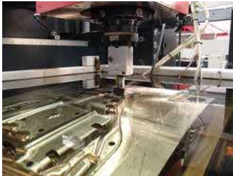
Gambar 65. Mesin EDM ( Electrical Discharge Machining )
