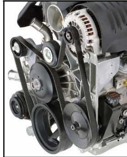
Gambar 5.4 Alternator Mobil
