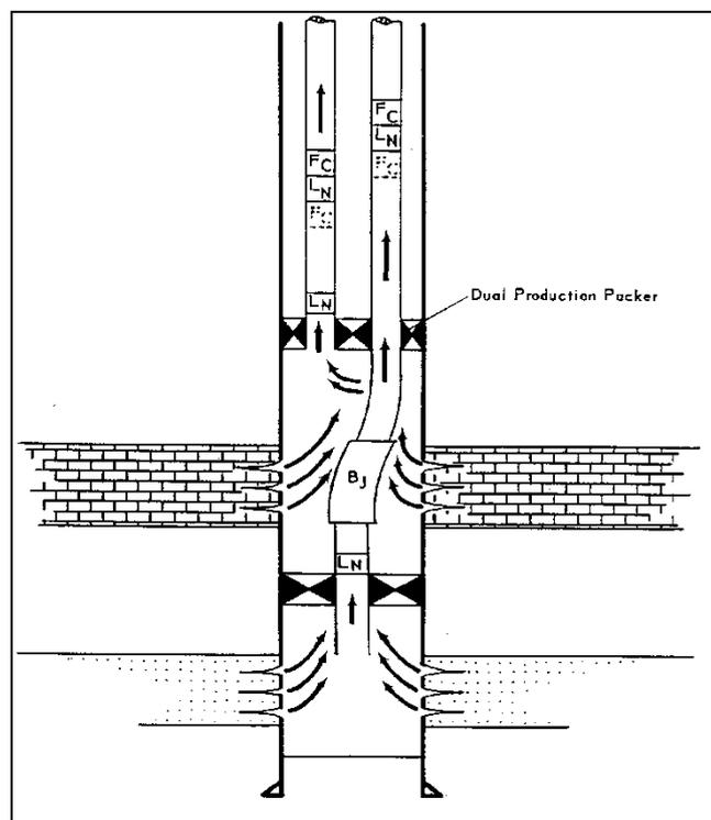
Gambar 6.3. Multiple Completion
