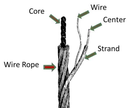
Gambar 4.9. *Drilling Line*
