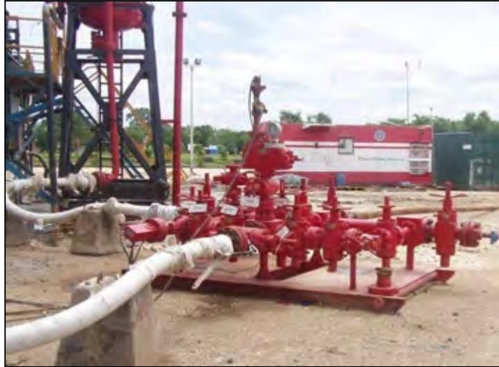
Gambar 4.44. *Choke Manifold*
