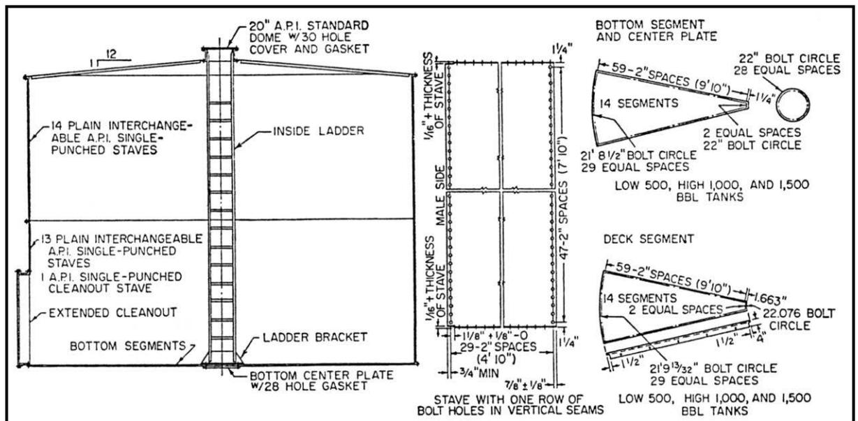
Gambar 8.23. Penampang Storage Tank Jenis Bolted-Steel Tank
