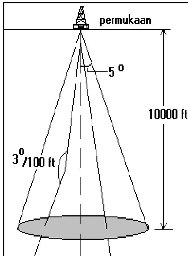
Gambar 3.6. *Straight Hole Drilling*
