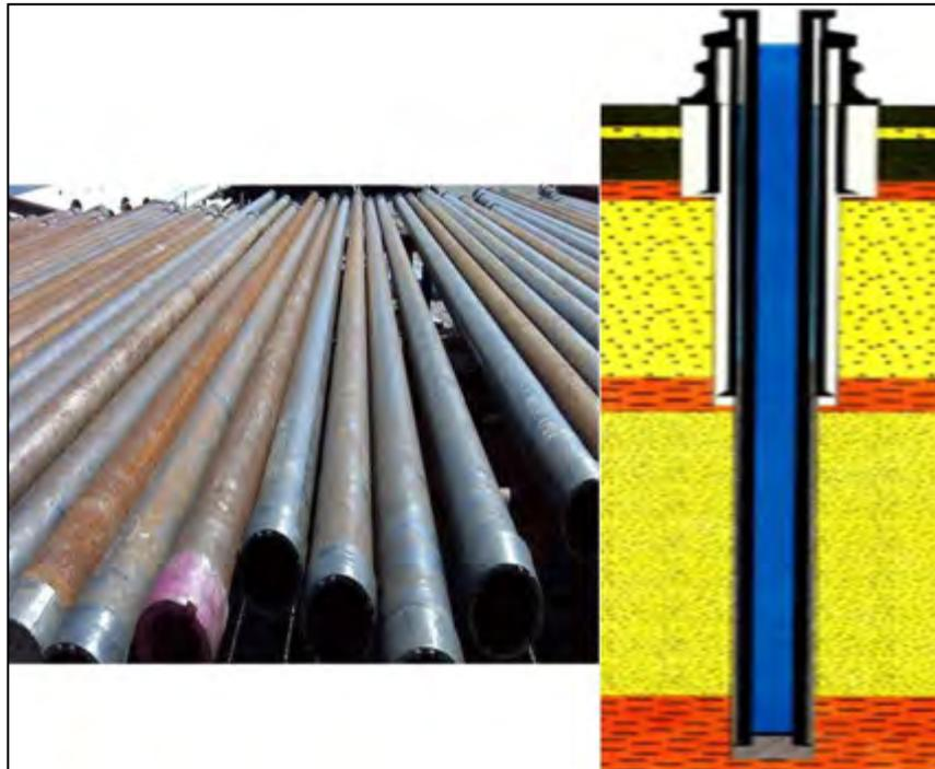
Gambar 5.4. *Intermediate Casing*
