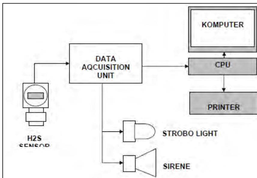
Gambar H<sub>2</sub>S Fixed Monitoring System
