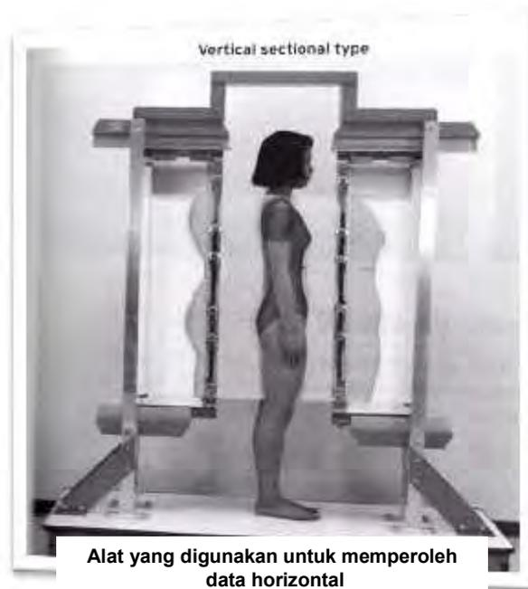
Gambar 2.13 *Sliding gauge measurement method*
