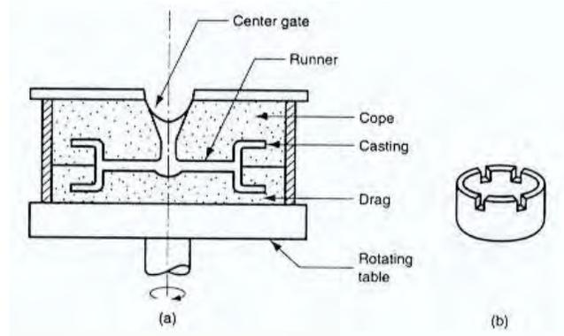
**Gambar 88. Proses pengecoran sentrifuge**
