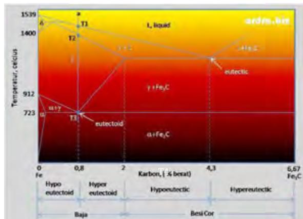
**Gambar 28. Diagram fasa besi karbida**
