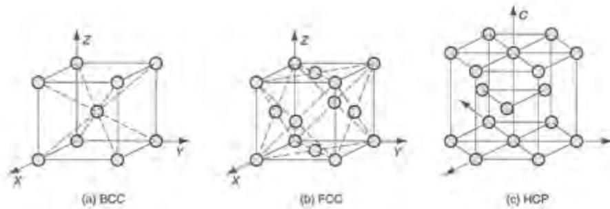
**Gambar 20. Tiga jenis struktur kristal logam: (a) *body-centered cubic*, (b) *face-centered cubic*, dan (c) *hexagonal-closed packet*.**
