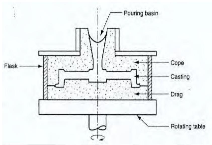
**Gambar 87. Proses pengecoran semi sentrifugal
