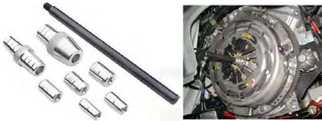
Gambar 4.5. Clutch Aligning Tool
