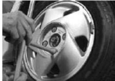
Gambar 2.20. *Over Tighten*
