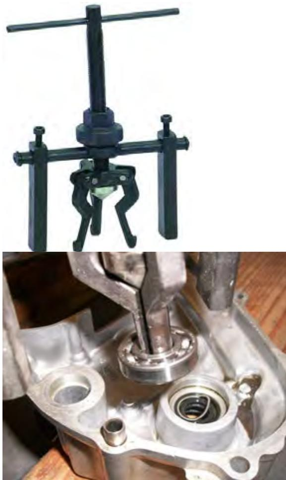
Gambar 4.3. Puller Bantalan Pilot (*Bearing Cup Puller*)
