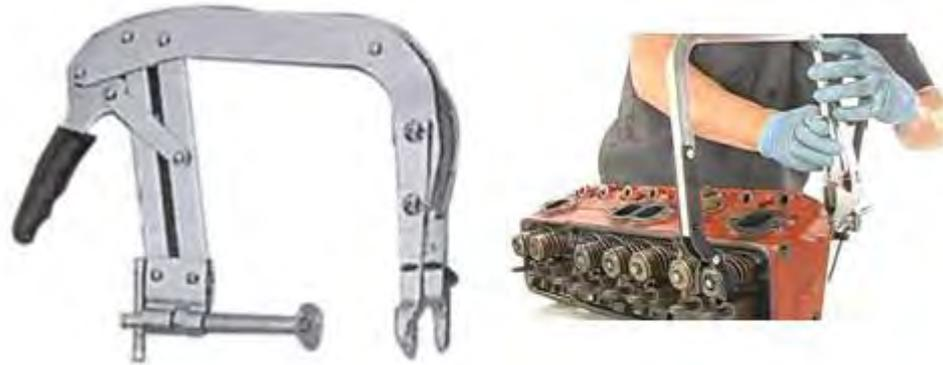
Gambar 4.13. Valve Spring Compressor
