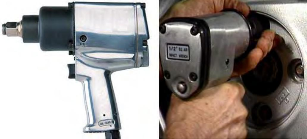
Gambar 2.17. *Portable Impact Wrench*
