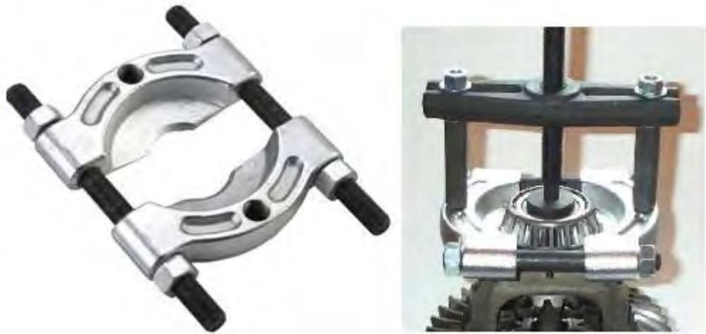
Gambar 4.1. *Bearing puller attachment*
