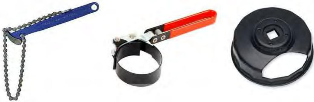
Gambar 4.14. Kunci Filter Oli (*Filter Strap Wrench*)
