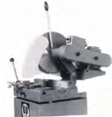
Gambar 2.45. *Cold Circular Saw*
