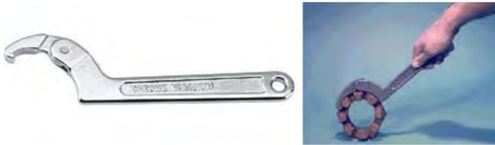
Gambar 4.22. Adjustable C Spanner / Fixed C Spanner
