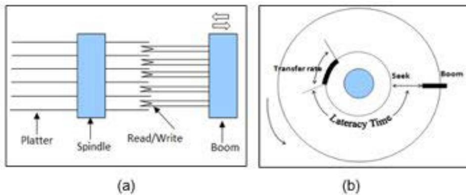
Gambar 50. (a) Struktur Disk (b) Proses seek disk
