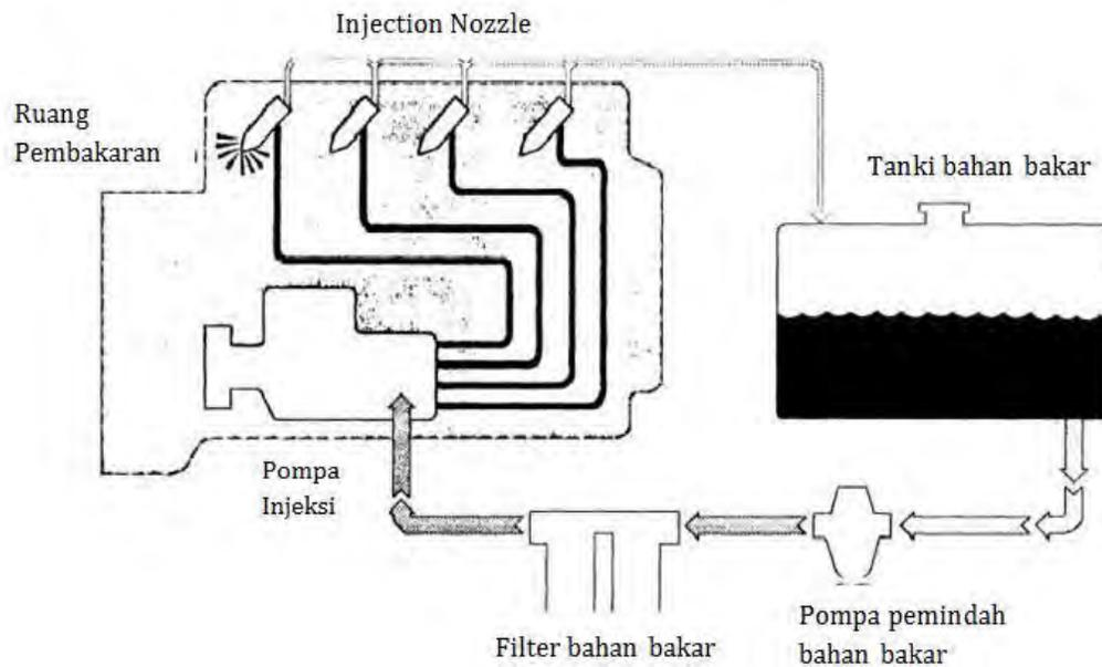
**Gambar 3. Skema sistem bahan bakar motor diesel konvensional**
