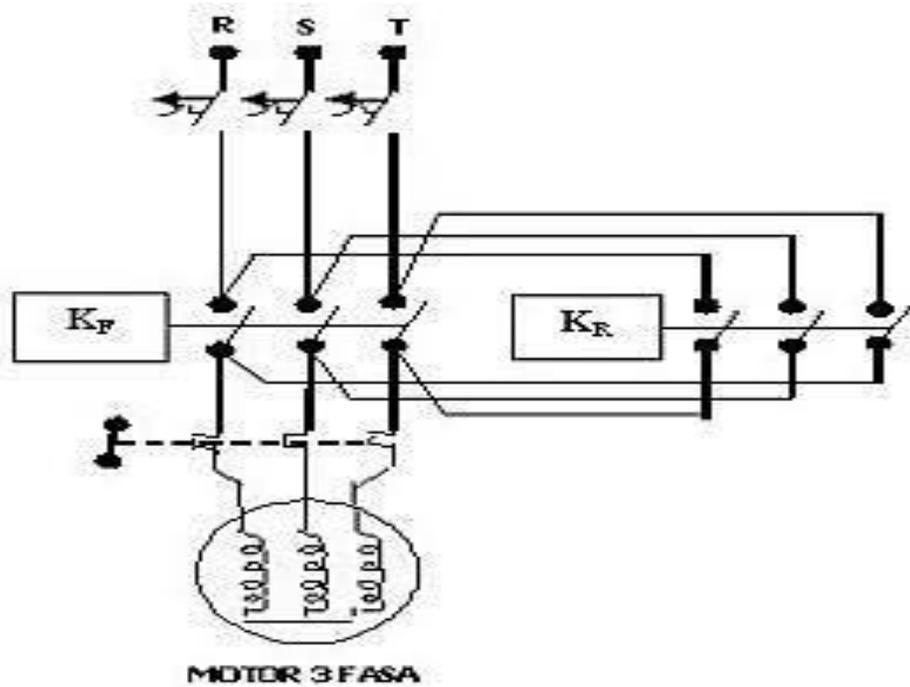
Gambar 38. Rangkaian 3 fasa putar kanan-kiri (*forward-reverse*) otomatis
