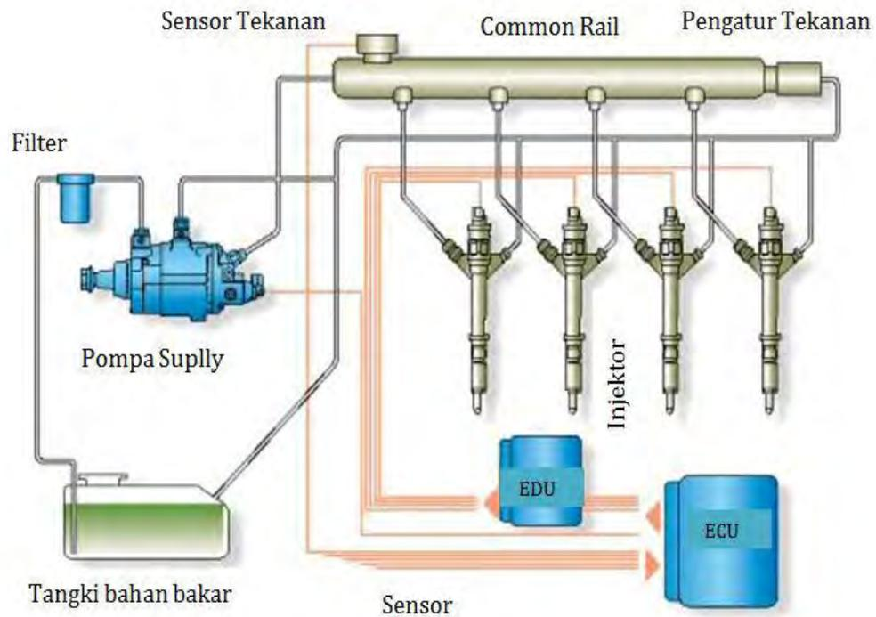
**Gambar 4. Skema bahan bakar diesel *Common rail***
