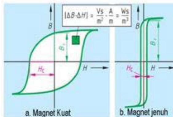
Gambar 2.25: Histerisis magnet permanen-ferromagnetik
