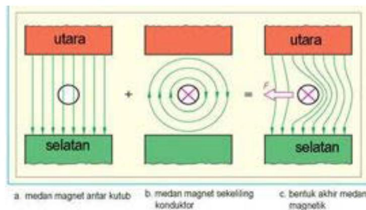
Gambar 2.28: Prinsip timbulnya torsi motor DC
