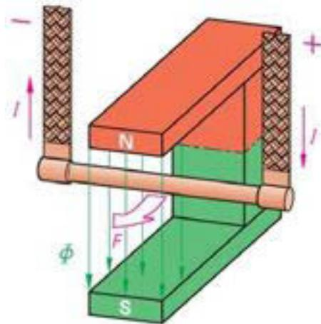
Gambar 2.27: Prinsip dasar motor DC
