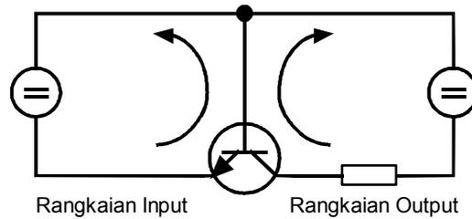
Gambar 8.12 Rangkaian Input-Output Transistor
