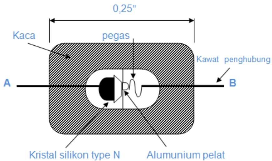
Gambar 7.2 Konstruksi junction dioda
