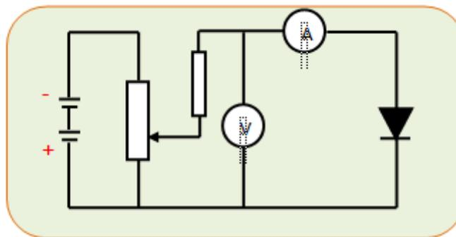
Gambar 7.8 Rangkaian dioda reverse bias
