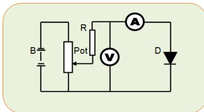
Gambar 7.7 Rangkaian dioda forward
