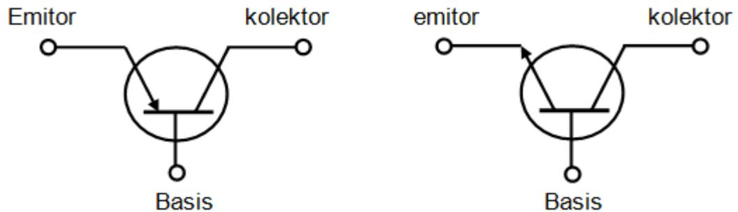
Gambar 8.3 Simbol Transistor
