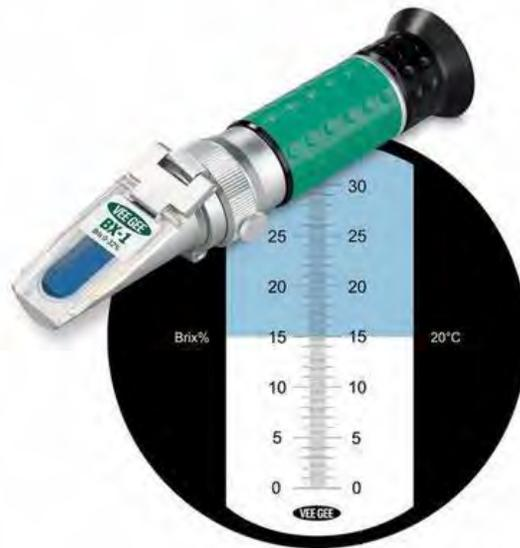
**Gambar 4. Hand Refratometer brik 0 – 32%**
