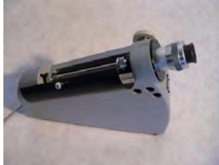
**Gambar 12. Zeiss polarimeter**
