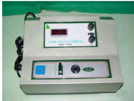
**Gambar 26. 1.0 ml Digital Photo Colorimeter (Model no. KCD - 10D)**
