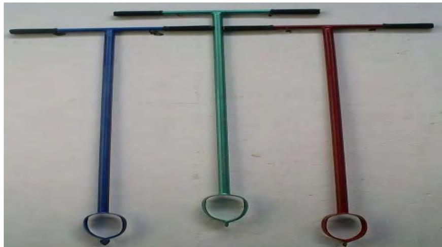
**Gambar 81. Alat/bor biopori model biasa**
