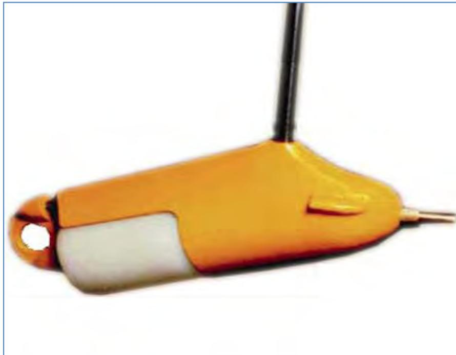
**Gambar 21. Depth 48 integrating sampler**
