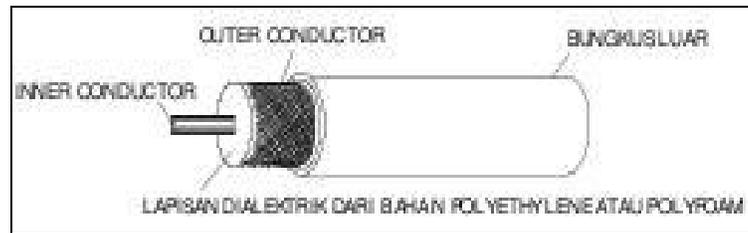
**Gambar 42. Bagian Kabel**
