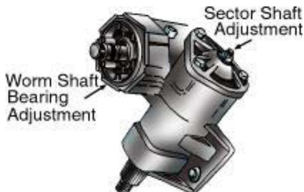
Gambar 174. Steering gear box.
