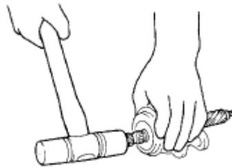
Melepas lower oil seal / pinion dan valve assembly.
