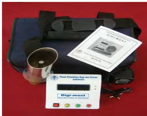
**Gambar 37. Alat pengukur kadar air/*Digimost* (iccri.net)**
