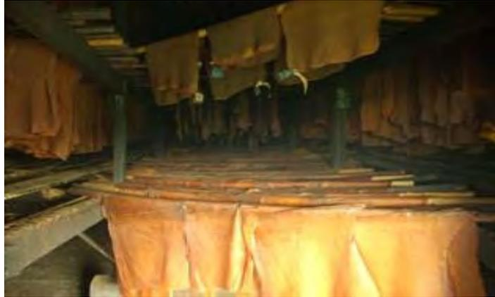
**Gambar 66. Proses pengasapan sheet**
