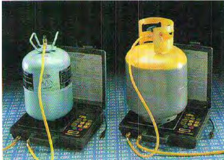
Gambar 5.9 Refrigerant Charging v.s Refrigerant Recovery
