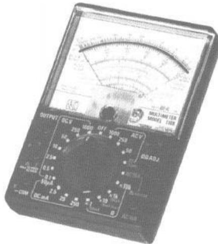
Gambar 4. 9 Multimeter analog
