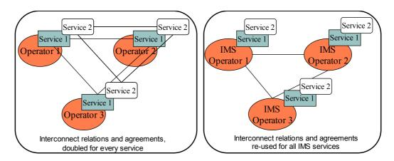
Figure 3. The difference in service interoperability between a pre-IMS network and IMS enabled operators
