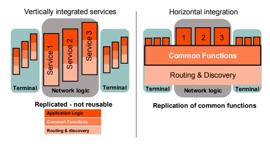
Figure 2. How IMS enables the move from vertical 'stove-pipe' service implementations to a horizontally layered architecture with common functions.
