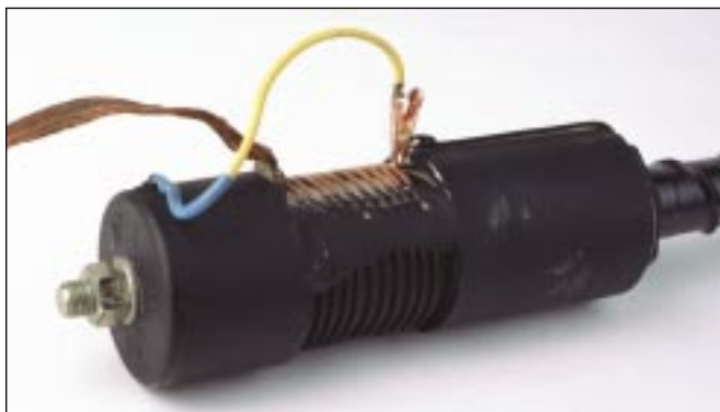
Close-up view of the matching coil. To the left is the \frac{3}{8} -24 mounting bolt. Attached to the bottom turn of the coil is a length of shield braid used as a ground strap. A small area of the PVC pipe OD is ground flat to provide room between the coil turns and the pipe form for an alligator-clip tap to firmly grasp a wire turn without interference.
