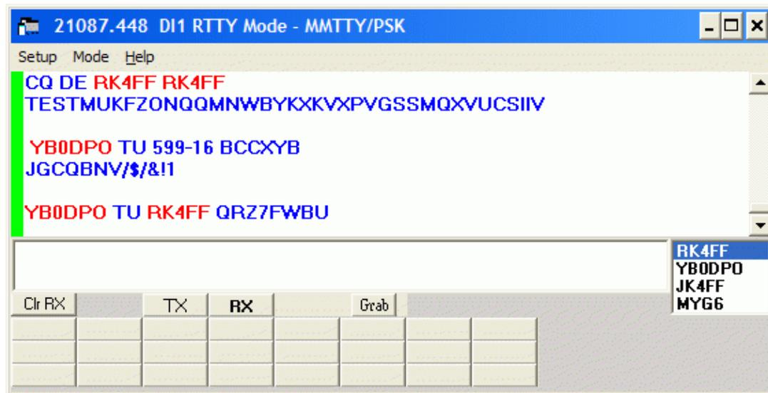
This is the Interface using MMTTY RTTY Engine. The Digital Interface is shown when it is selected under Window in the Entry Window.
